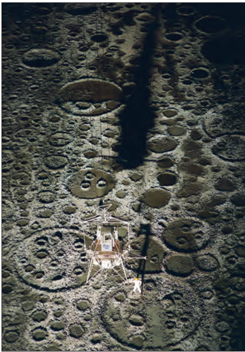
Apollo astronauts practiced for lunar missions at NASA Langley's Lunar Landing Research Facility. This 1969 photo of the facility shows its model Lunar Excursion Module, or LEM. The LEM was suspended from cables to enable the astronauts to simulate piloting on the moon. A Langley worker is standing beneath the craft.
