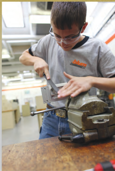
John Stuttz, 19, files a spare part for a computer controlled milling machine at Blum Inc. He is in his third apprenticeship year.
